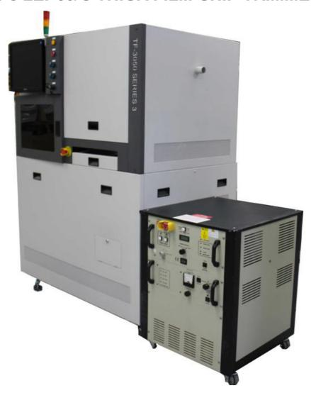
The **TF-3050 Series 3 LEP60/C** provides high accuracy performance to overcome the new challenges of smaller geometries of chip resistor trimming. Proprietary designs achieve the high accuracy mechanical positioning and ultra-stable laser beam control demanded by industry. **TF-3050 S3** utilizes vision registration theta rotation within a Windows XP operating system. These advance features are integrated with established substrate handling and automation systems.
